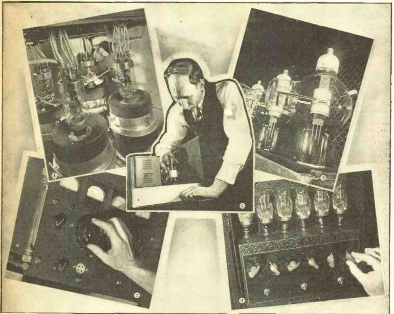
Symbols of modern radio and industry! Photo (1) shows four of the big air-cooled 50,000-watt modulating tubes used in a large broadcasting station. Two of these are spares or "standbys." Simply by pushing a button the operator can put them into service without removing defective tubes or interrupting the transmission. The center photo (2) shows the special moisture-detecting tube going into place in an electronic installation for control of moisture in a manufacturing process. The photo at the upper right (3) shows U.H.F. tubes used in inter-continent communications. Photo at the lower right (4) gives some idea of the appearance of a precision electronic timer, which automatically divides the time required for a spot-weld, into fractions of a second. Photo (5) shows the hand of an operator setting the adjustments on an electronic furnace control, which provides high efficiency, not obtainable by other means. —Photos, Courtesy of Westinghouse.
